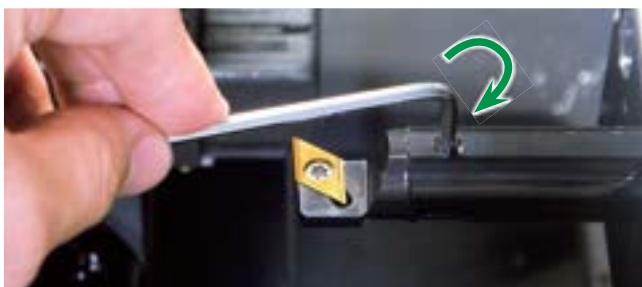
3. Raise the center height by one half of the dia. of the boss.
